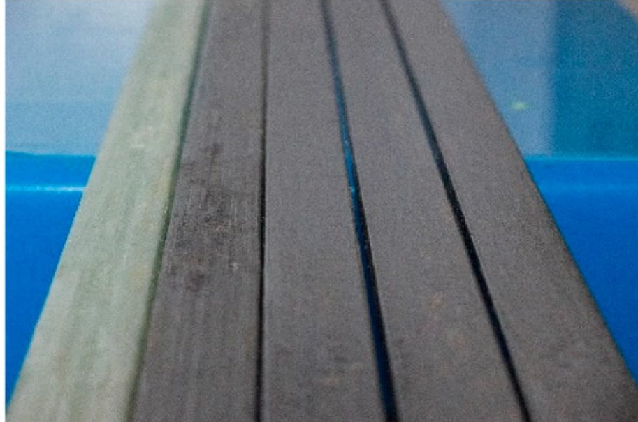
Figure 2. Optimized bio-based polyester and basalt fibers profile obtained by pultrusion (20 yarns of basalt fiber). Samples in AIMPLAS' facilities.
