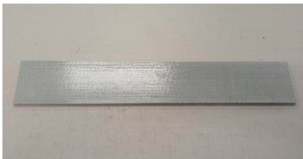
Figure 4. Bio-based polyester and glass fiber profile obtained by pultrusion obtained in OMIKRON's facilities.
