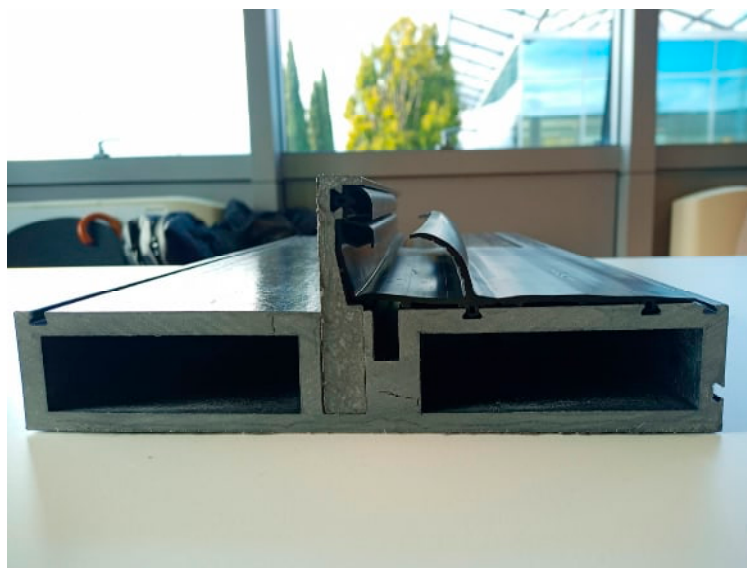
Figure 3. Image of the bio-based pultruded profile tested.
