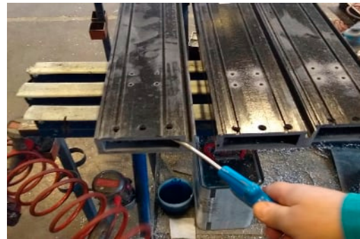
Figure 6. Dust removal after the machining phase.
