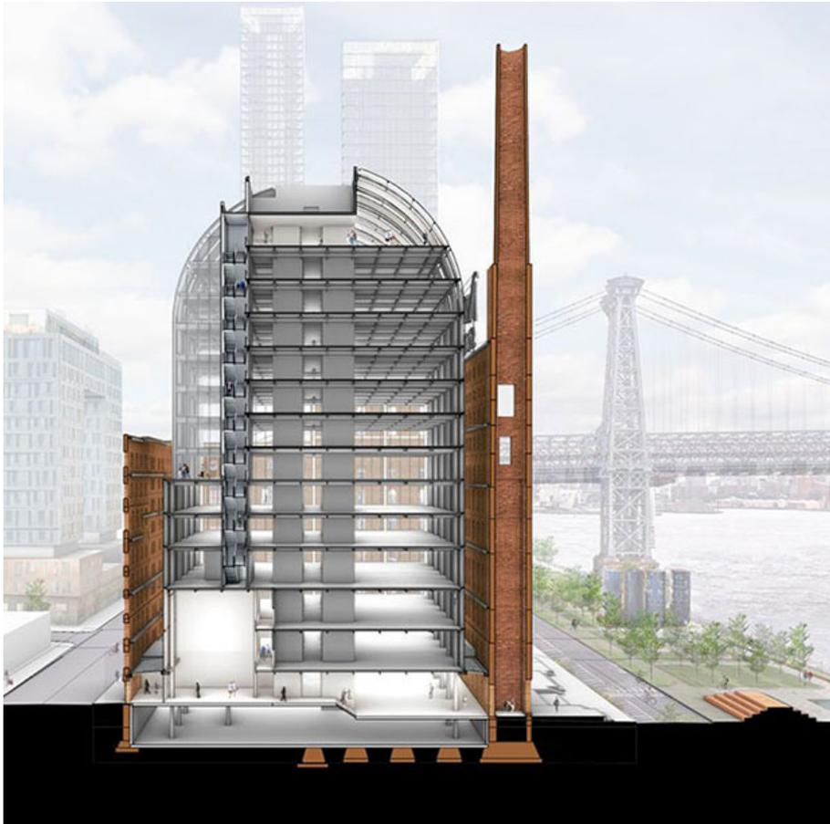
↑ Section of the project. You can see the space between the exterior walls and the new internal construction.
