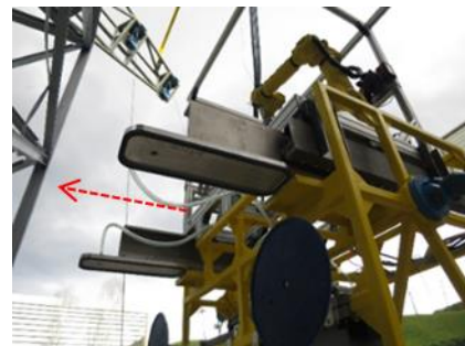
Figure 4. Stabilizer of the robot's frame prototype during the opening of the stabilizers.
