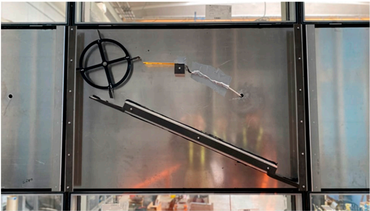
Figure 11. The PE-EHS cantilever, configured within the wheel setup, installed in the façade within a laboratory testing facility. The airflow within the cavity triggers the rotation of the wheel, and the magnets positioned at its extremities generate a magnetic force with the magnet located at the end of the PE cantilever, thereby enabling vibration.
