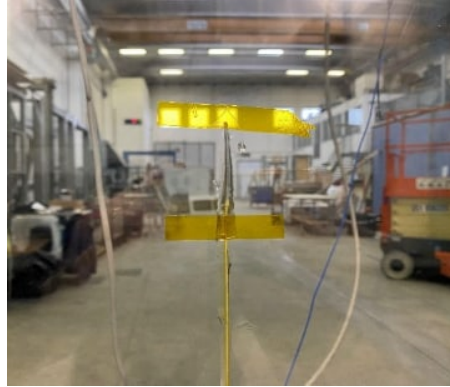
Figure 9. FBGs sensors applied on the glass surface for temperature monitoring.
