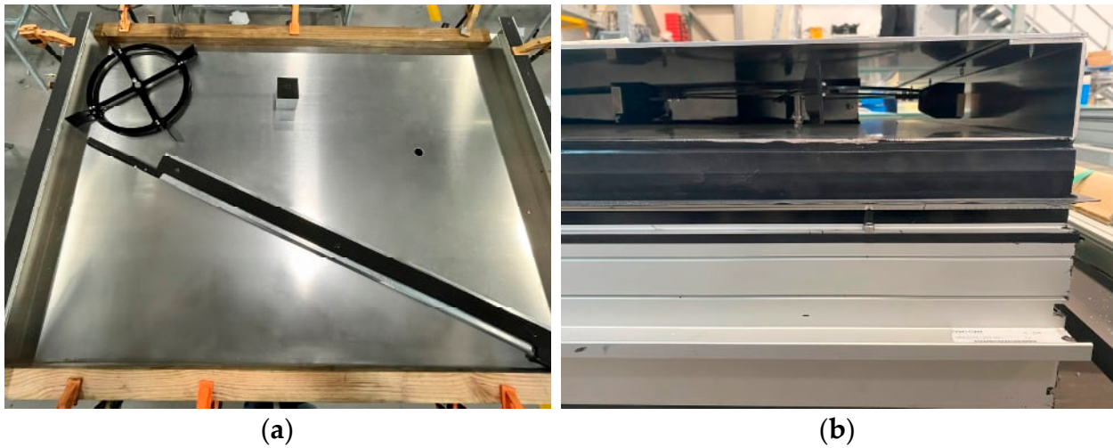
Figure 10. EP-EHS wheel configuration installed in the façade: metal sheet cladding with an air channel and wheel integrated (a); EP-EHS wheel configuration's ventilated air cavity in the façade (b).
